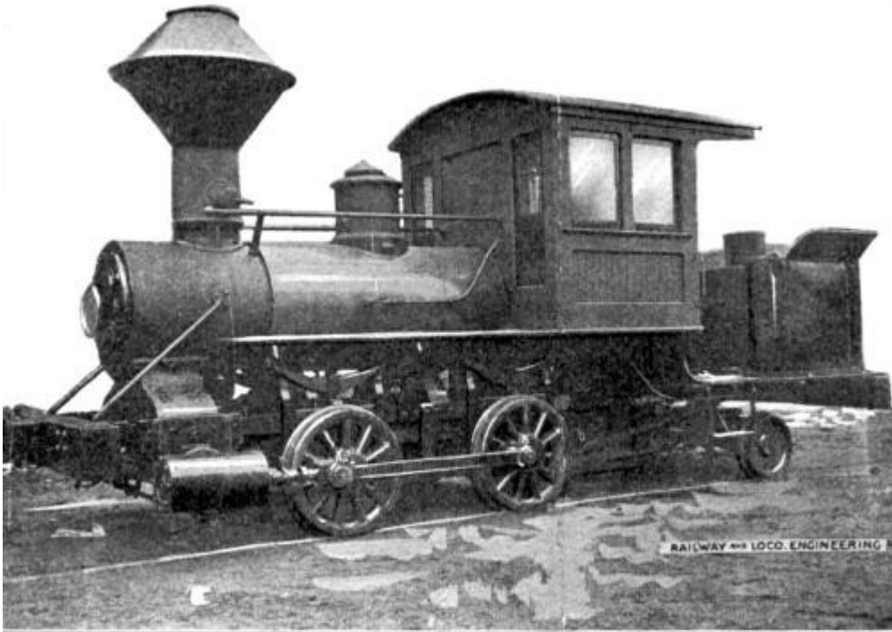
FIG. 30. ENGINE WITH OSCILLATING CYLINDER AND NO VALVE GEAR.
